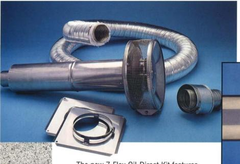
The one-piece vent section is comprised of an airtight, watertight, 316 titanium flexible tube, wrapped with a high temperature insulation blanket, and a 2-ply flexible aluminum jacket.
